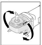
The machine head can be rotated with respect to the machine housing in 90° steps. In this manner, the On/Off switch can be brought into a more convenient position for special working situations, e.g. for lefthanded persons.
