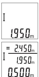
To switch on the laser beam, briefly press the measuring button **2**. To initiate another measurement, briefly press the measuring button **2** again. The current measured value **c** is displayed in the bottom line. The previous measured value **b** is displayed in the middle line. In the top line, the auto-sum **a** (the sum of the current and previous measured value) is displayed.
