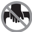
Never carry the power tool using the handle of the glide arm.
